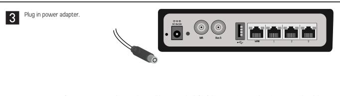
QUICK TIP: To **soft reset** your router, depress the small button to the left of the power input with a pin or paper clip while the unit is powered on.
